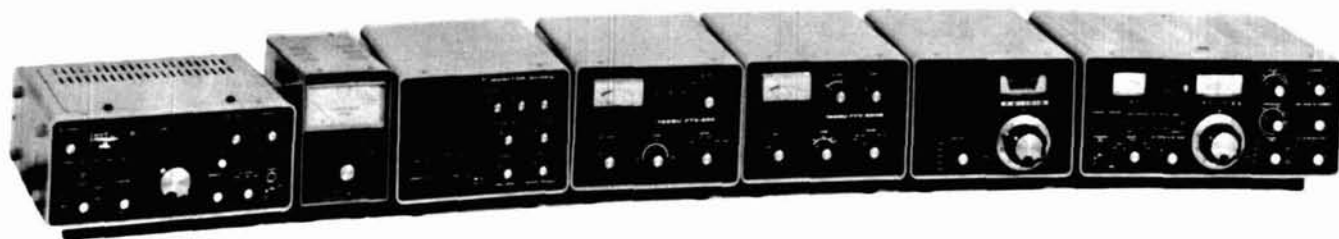
Left to right - FT-620B, 6 Meter Transceiver • YP-150, Dummy Load Wattmeter • YO-100, Monitor Scope • FTV-250, 2 Meter Transverter • FTV-650, 6 Meter Transverter • FV-101B, External VFO • FT-101E 160-10 M Transceiver
